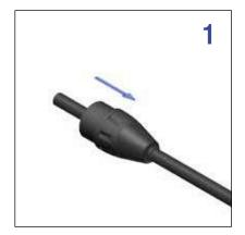
Slide the nut (Backshell) onto the cable
