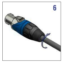
Thread the nut onto the shell to activate the cable clamp and close the connector assembly.
