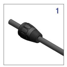
Slide the nut onto the cable
