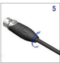
Thread the nut (Backshell) onto the shell (Torque 0.8Nm - 1.2Nm) to activate the cable clamp and close the connector assembly.
