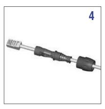
Close clamp-boot, fasten the two tabs together to lock.
