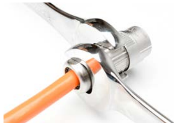
Step 17 - Tighten to 5-7 N/M using 25mm wrench
