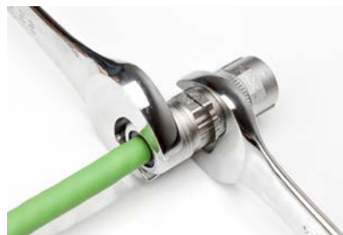
Step 16 - Tighten to 5-7 N/M using 25mm wrench
