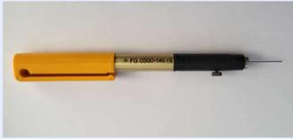
1. Extend the pin out of the release tool and fix it in place
