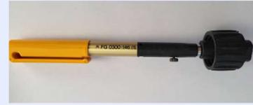
3. When fully inserted pin or socket contact can be pulled out with slight force
