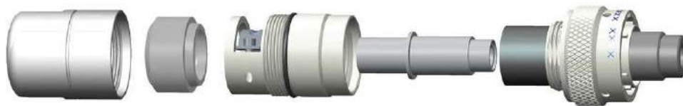
Step 1: Slide components onto cable
