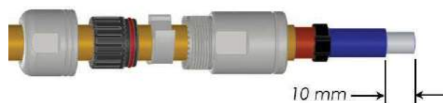
Step 6: Slide plug onto crimped terminal assembly
