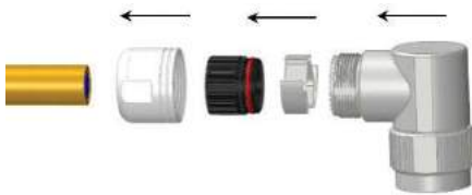
Step 1: Slide parts onto cable
