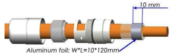
Step 4: Wrap foil over braided shielding
