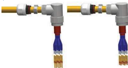
Step 7: Attach contacts to wire leads
