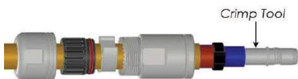
Step 5: Crimp terminal to conductor
