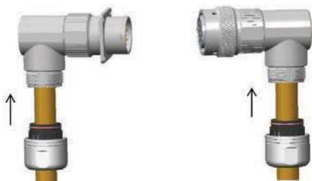
Step 11: Push shielding clip into backshell
