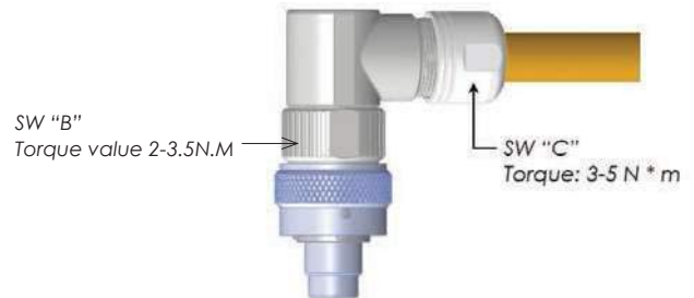
Step 12: Attach cable-nut to backshell and tighten as shown
