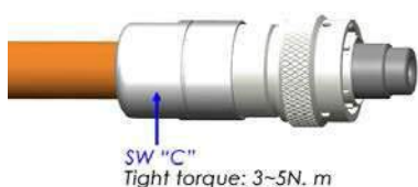
Step 9: Attach and tighten backshell as shown
