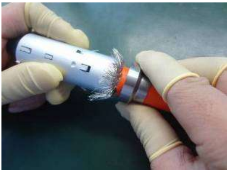
屏蔽铜丝向前翻到金属屏蔽套上 Shield wire forward turn to metal shielding
