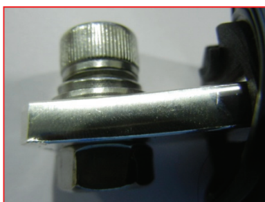
f、 检查胶料是否破损，检查PIN是否弯曲变形 Any damage on plastic is not allowed, any deformation on Pin is not allowed.
